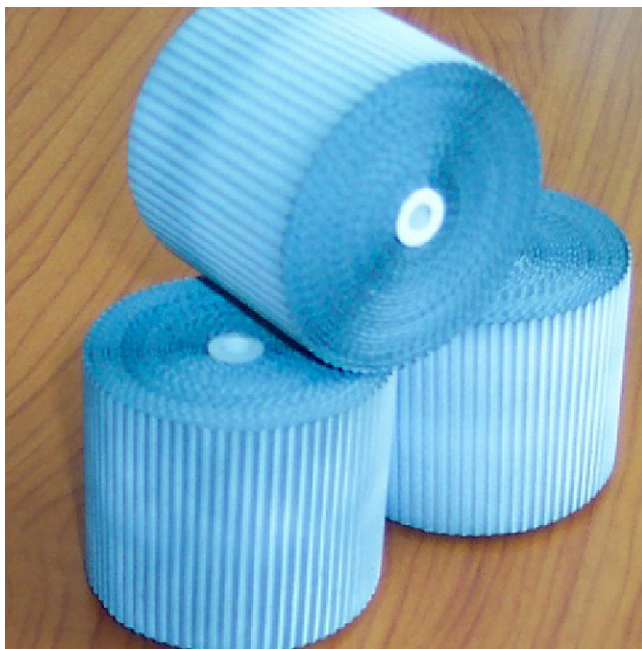
Fig. 2. A view of metallic catalyst supports used in the experiments.
